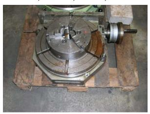
Index and Turntable Mauser-Bruche; Serial No: 1002; Table Ø 500 mm; 7 T-Slots horizontal/vertical use.
