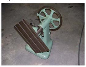
Turn table horizontal / vertical use; Ø 400 mm; 6 T-Slots; 3Jam Roehm Ø 250 chuck
